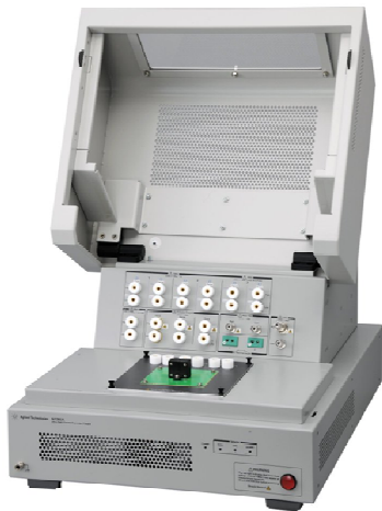
Figures 1-2. Agilent N1265A UHC Expander/Fixture.
